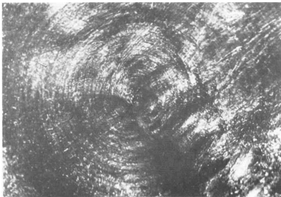
FIGURE 4 A rotational structure of CLC motion at the tip of a slip band. Polarized light.
