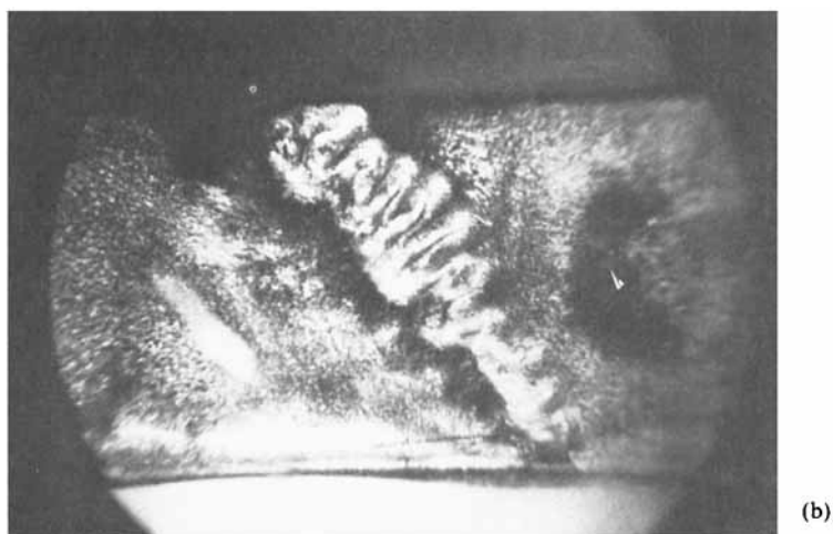
FIGURE 1 The structure of convective motion in CLC layer over a slip band during deformation of a NaCl single crystal. Unpolarized light. \times 20 . a) the onset of CLC movement causes a distortion of the initial texture of the CLC layer; b) a spiral structure of CLC motion; c) a residual picture of CLC motion observed in 1–3 min after the deformation had stopped; d) re-generation of a spiral structure after the deformation recommencing.
